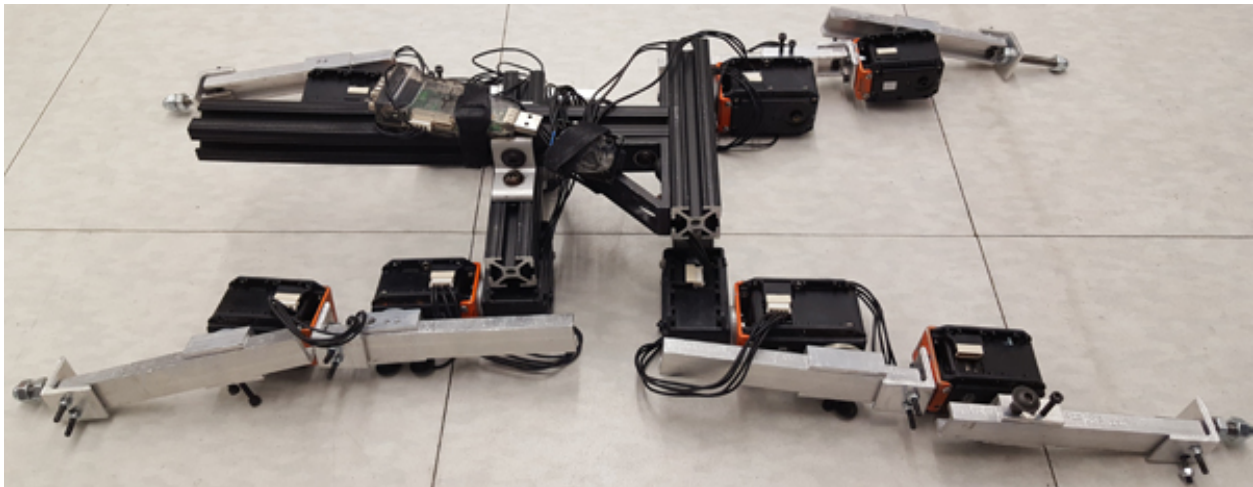
Figure 43: The reconfigurable robot in its initial small configuration.
